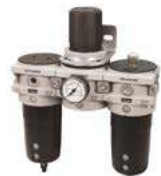
Combination Filter + Regulator + Lubricator, 12 bar, 5 micron
